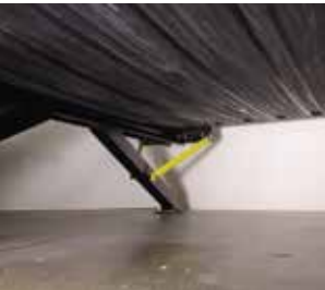
Electric Stabilizer Jacks W/Footpad - Make setup & teardown sweat free, keeping your trailer stabilized while parked. - N/A 1475 & 1575
